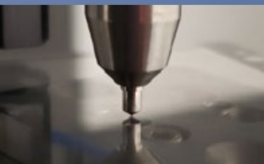
Scratch indenter in contact with a screen
