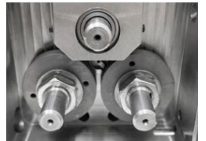
3 Rollers During Test
