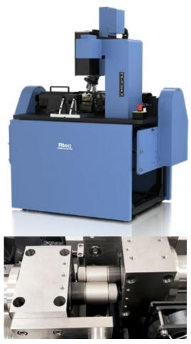
Two Roller During A Test
