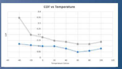
Two Sample COF vs. Temperature Comparison
