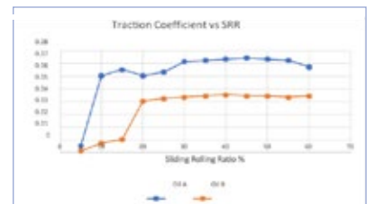
Traction Coefficient vs. SRR Test Results
