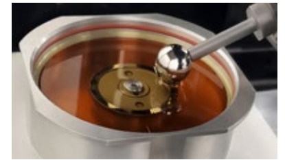
Traction Module and Sensor During a Test
