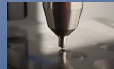
Scratch indenter in contact with a screen
