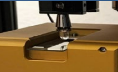
A test showing hydrogel against a coated glass slide. Real-time contact area analysis vs. force.
