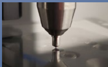
Scratch indenter in contact with a screen
